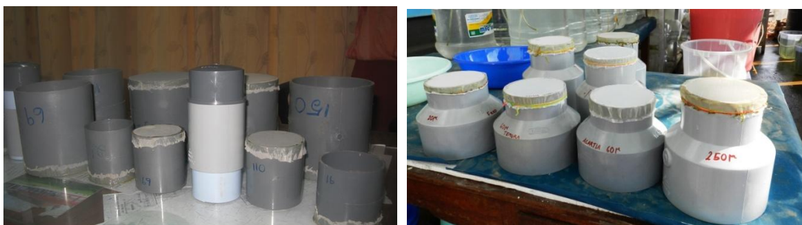
Sieves of different mesh sizes made from plastic pipe connectors and bolting silk
