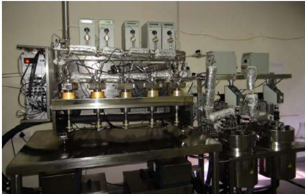
High pressure fermenter 350 bar pressure rated
