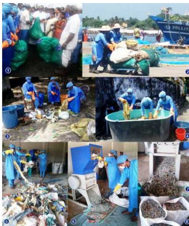
1. Receiving waste containing bags from boats; 2. Workers carrying the bags in trolleys to the segregation area; 3. Segregation of wastes; 4. Washing the plastic wastes; 5. Cleaned and dried wastes brought to the shredding unit; 6. Loading the plastic wastes into the shredding machine; 7. Shredded plastic product; 8. Stored in sacs for further use
