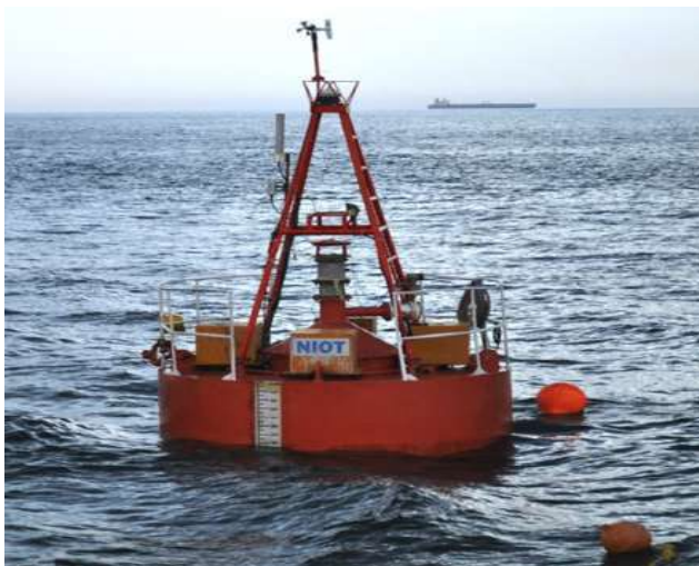
Wave powered Navigational buoy
