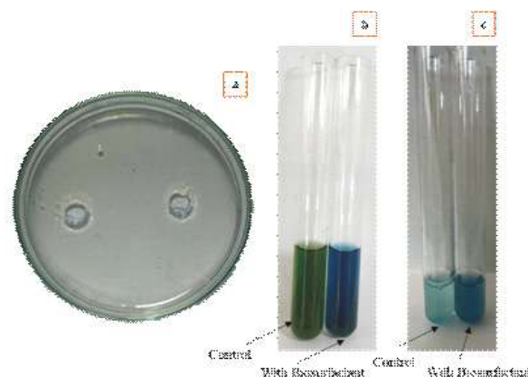
Figure 3. Identification of functional groups/bonds using a) Cetyl trimethyl ammonium bromide (CTAB)/methylene blue agar test, b) Bromothymol blue (BTB) test and c) Biuret test
