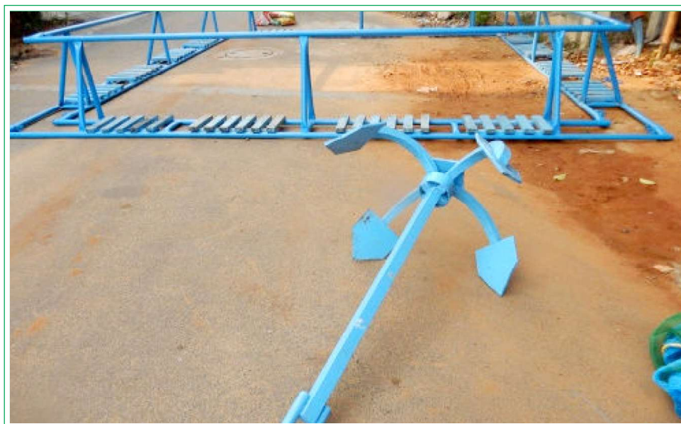
Fig.2: Structure of coastal cage and toothed anchors
