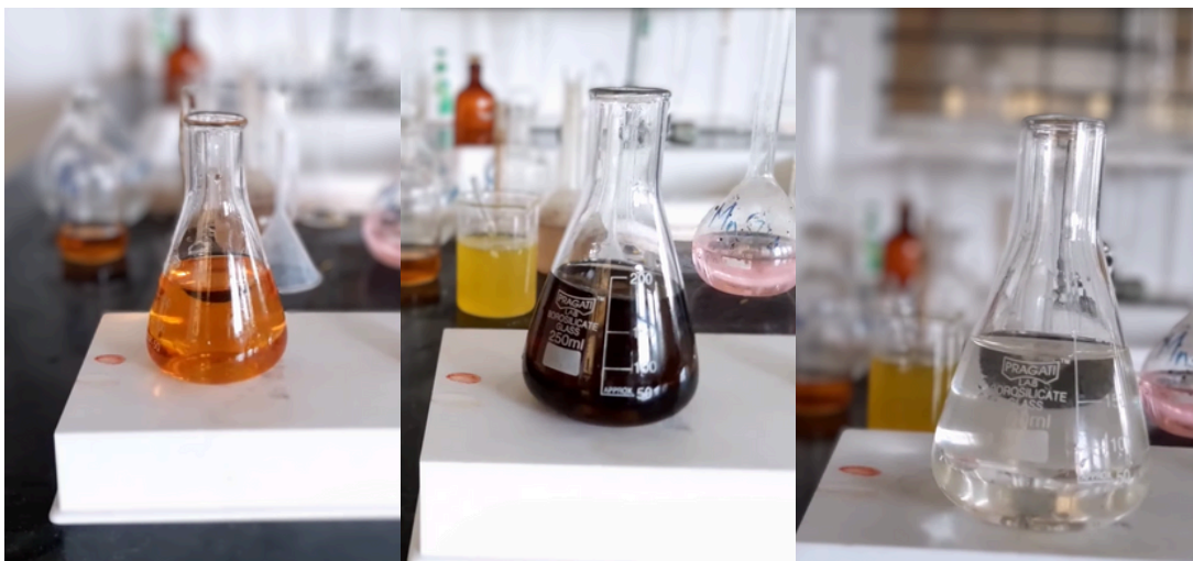
Fig 3.7 Gradual Color Change during titration
