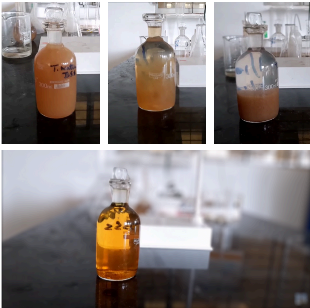
Fig. 3.6 Precipitation formation after adding Conc. Sulfuric Acid to the water sample
