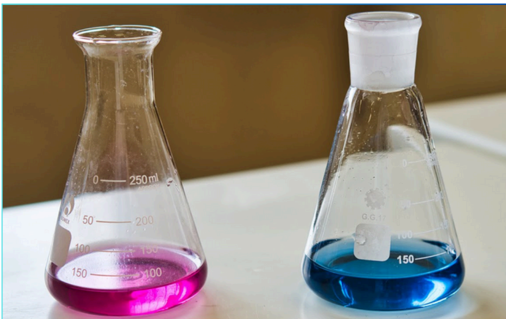
Fig. 5.1 Gradual change in colour during titration for hardness analysis
