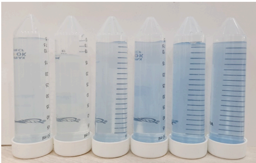
Fig. 4.12 Preparation of Silicate Standard Solutions at Different Concentrations for Spectrophotometric Analysis
