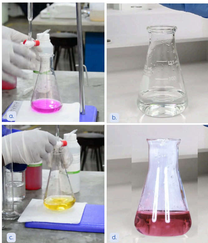
Fig 3.5 a. Sample after adding phenolphthalein indicator b. Sample after first titration, c. Sample after adding Methyl orange indicator, d. Final titration
