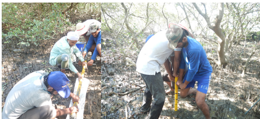
Sediment sampling using PVC core sampler
