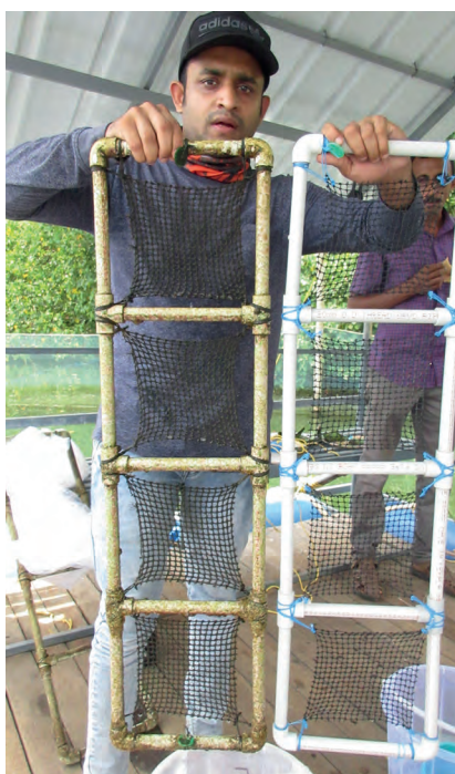
Experimental net panel before and after six months of anti-fouling trial
