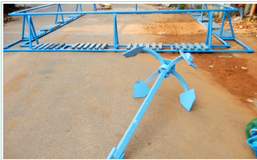
Fig.2: Structure of coastal cage and toothed anchors
