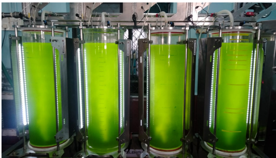
Photobioreactor based mass culture of microalgae
