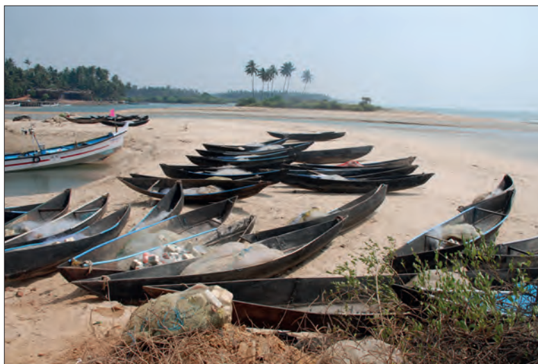
Plate 6. Dug-out canoes for coastal gillnet fishing
